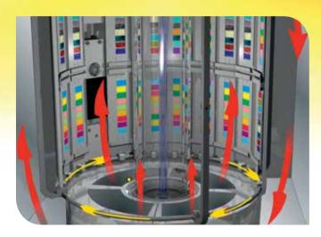
Air Flow in Test Chamber
